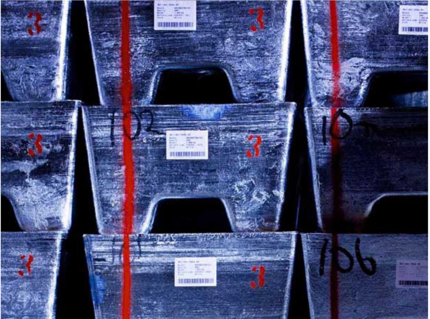
**ZINIGAL<sup>®</sup>**, a zinc-nickel alloy, was developed by Boliden to meet the needs of our customers in the general galvanising industry. The easy to use, ready-made alloy means no more mixing of different components, saving our customers time, effort and costs.
