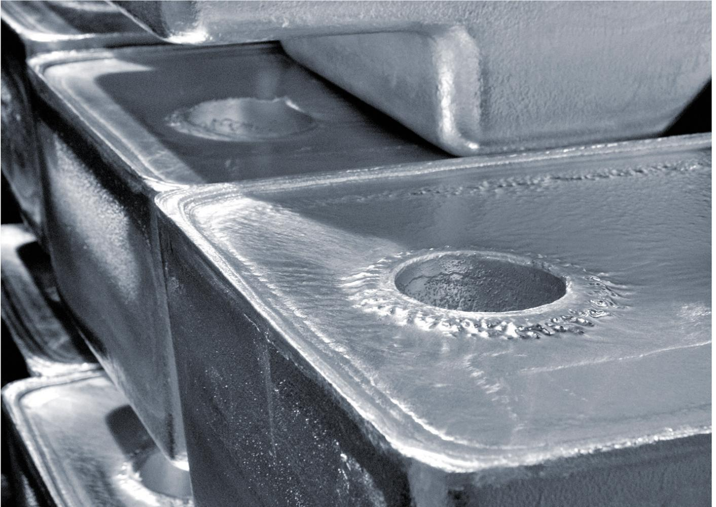
**ZINC-BRIGHT®**, a zinc-bismuth-tin alloy for Lead-free galvanizing, was developed by Boliden to meet the needs of our customers in the general galvanizing industry. The easy to use, ready-made alloy means no more mixing of different components, saving our customers time, effort and costs.
