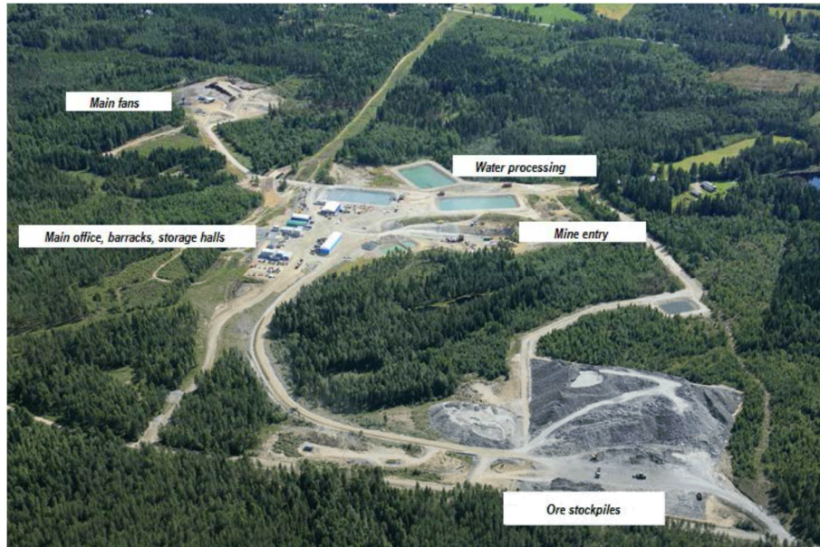
Figure 14. Surface infrastructure of Kylylahti mine.
