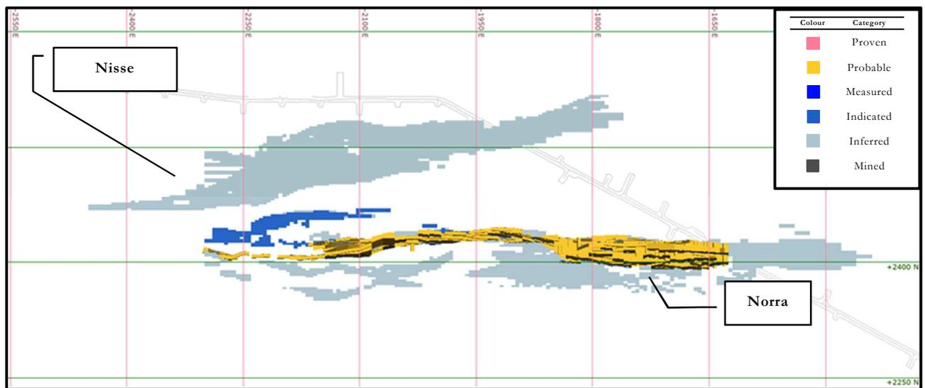
Figure 12. Plan view of the Rävliiden Norra Mineral Resources and Mineral Reserves.
