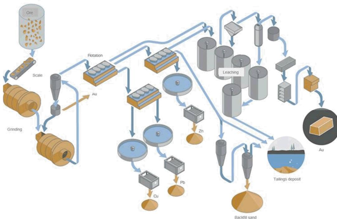
Figure 10. Schematic diagram of the Boliden Area Operations processing plant
