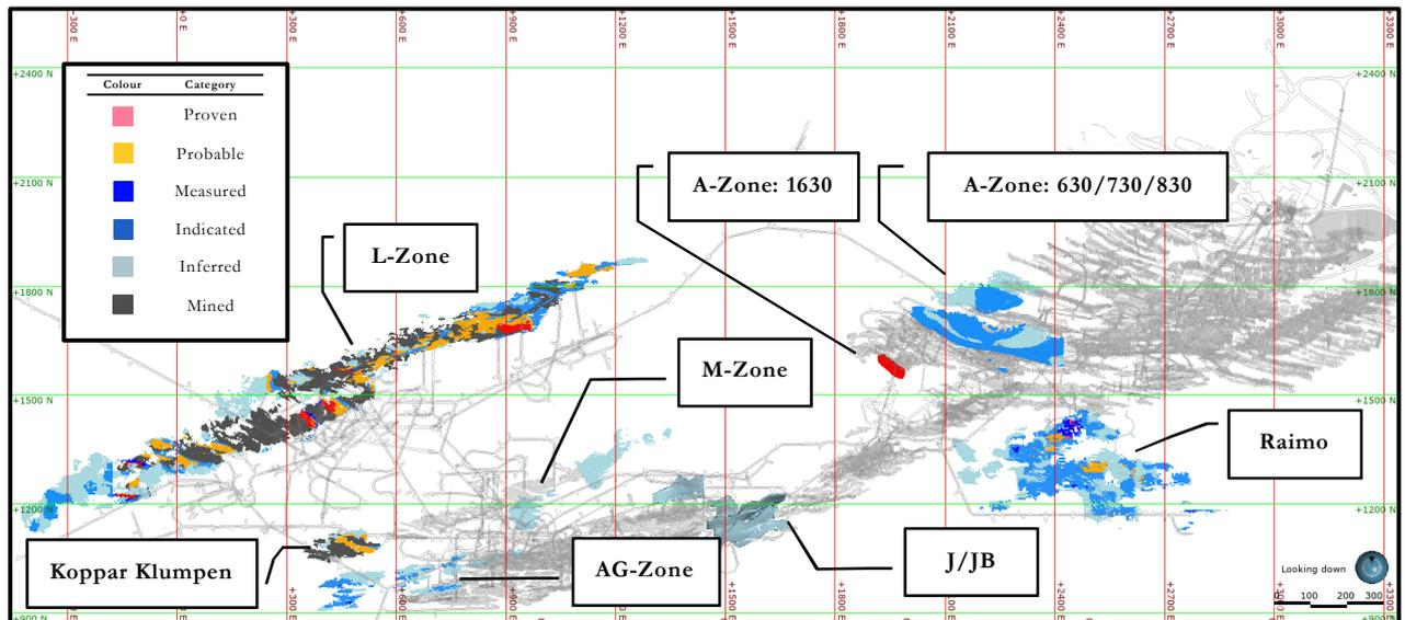
Figure 11. Plan view of the Kristineberg Mine showing mine infrastructure, historical mined areas and locations of Mineral Resources and Mineral Reserves
