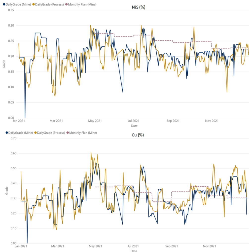
Figure 12. NiS and Cu grade comparison between grade control (Mine) and process (Process)
