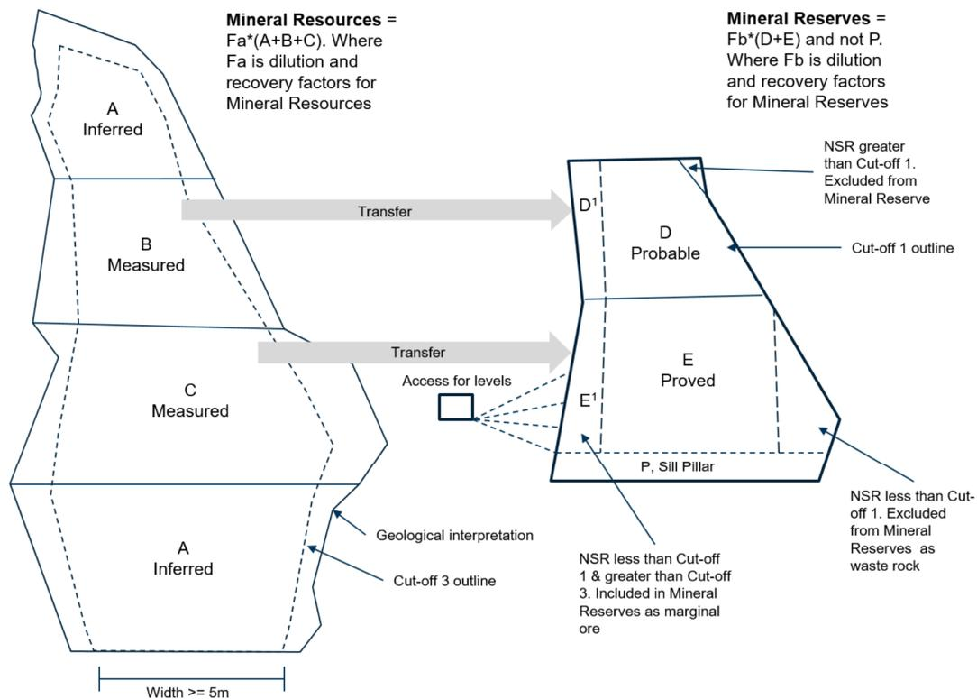
Figure 5: Schematic illustration of the principles for reporting of Mineral Resource and Mineral Reserve at Renström
