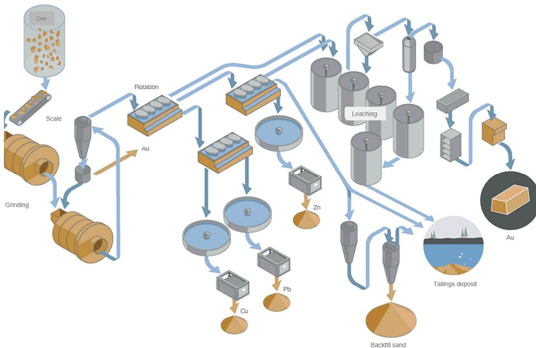
Figure 2: Simplified overview of the different stages of Renström ore processing at BAOPP
