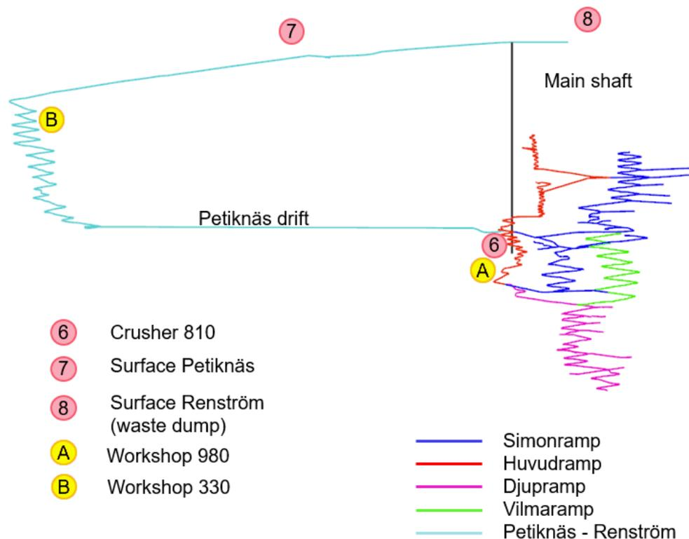
Figure 3: Schematic cross section of the Renström ramp system and Petiknäs decline with crusher and workshop location (looking due north. field of view ~3km horizontal & 1.5km vertical).
