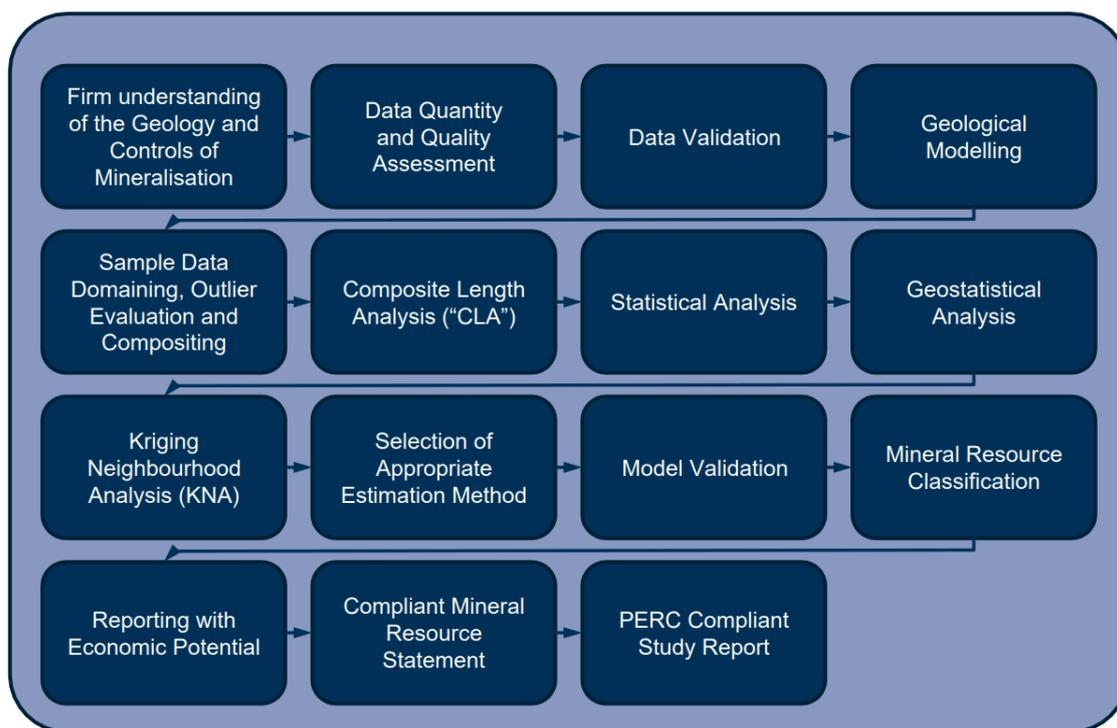
Figure 4: Ore Reserves and Project Evaluation group Mineral Resource estimation workflow
