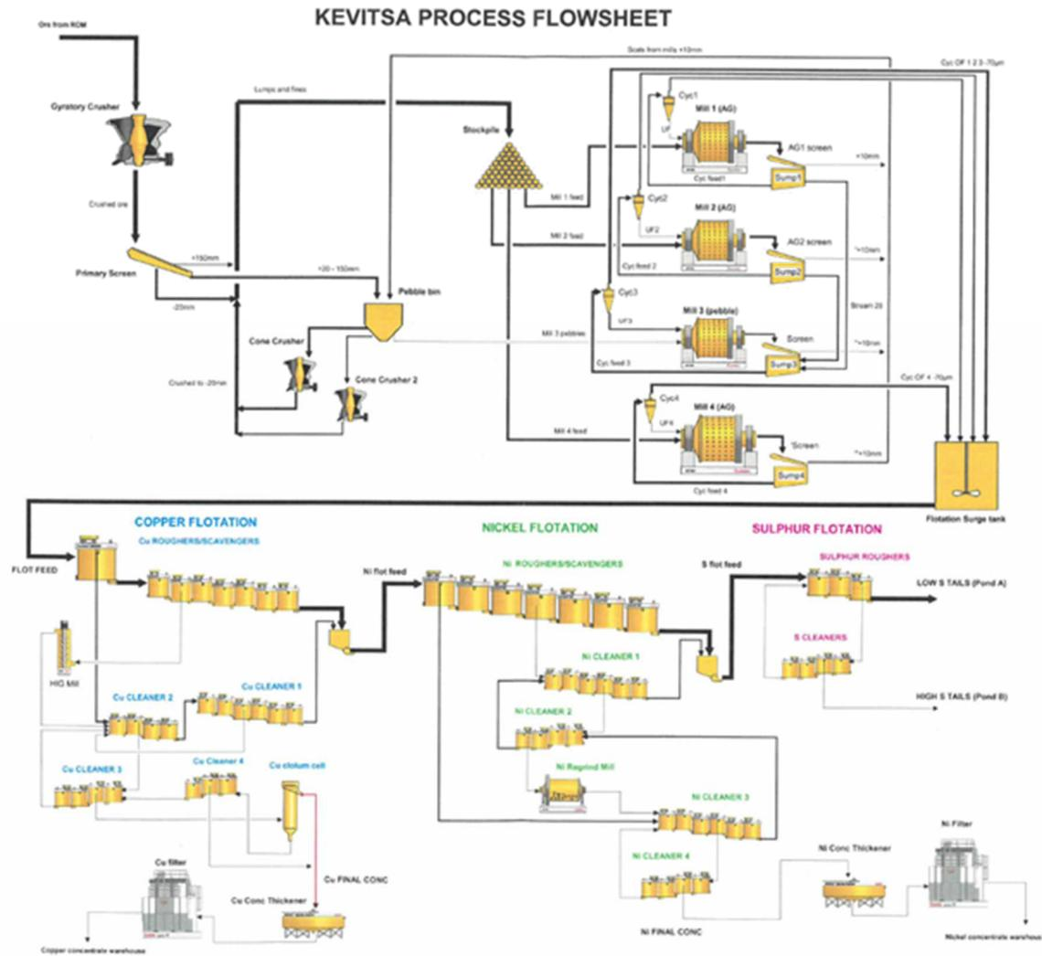
Figure 7. Simplified flowchart of the Kevitsa Mine process
