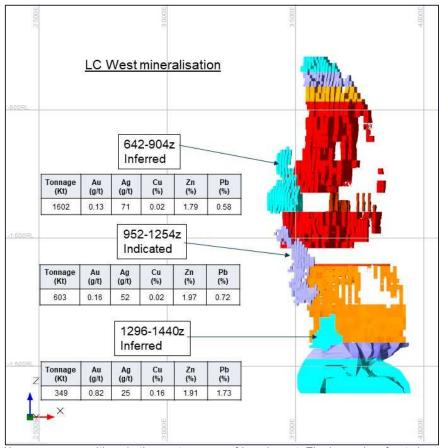
Figure 3-11. New resource positions in the western area of Lappberget. The image is a front view of Lappberget ore body, looking north.
