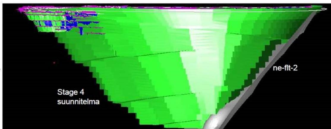
**Figure 14-13: Stage 4 pit design with NE-FLT-2 Structure located near east wall**
