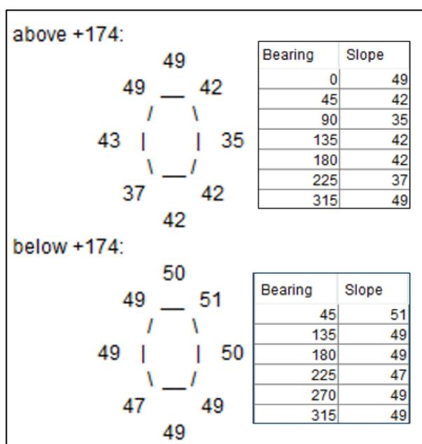
**Figure 14-1: Radial overall slope angles – geotechnical input parameters**
