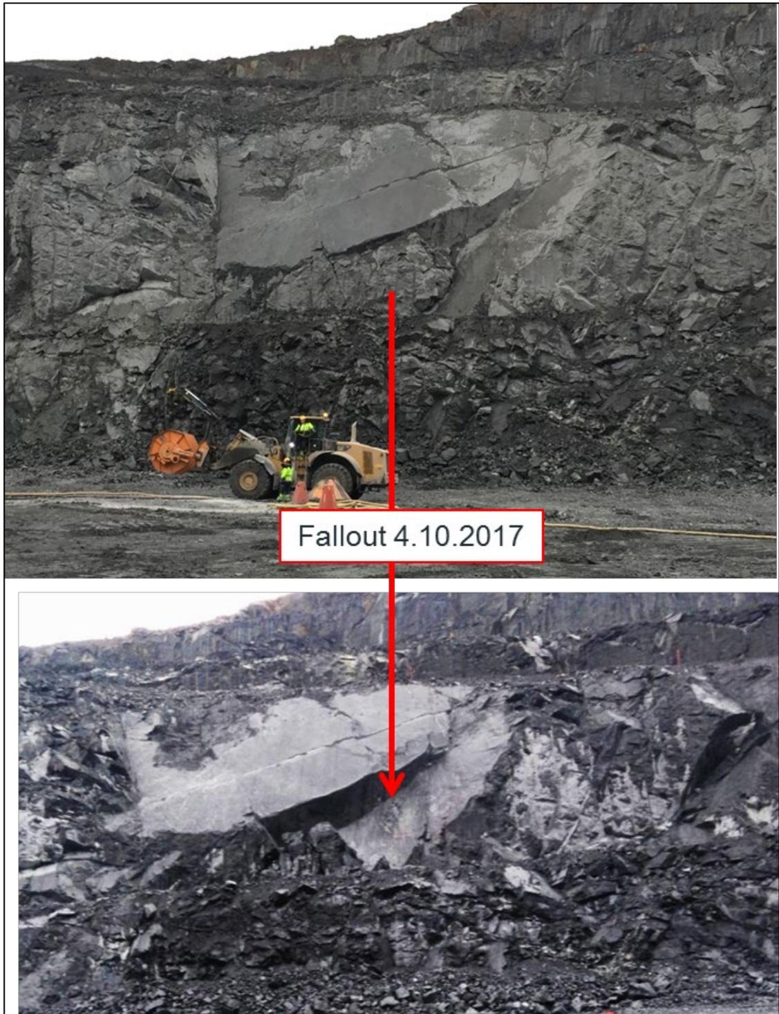
**Figure 14-14: Example of typical bench scale wedge or planar failures**
