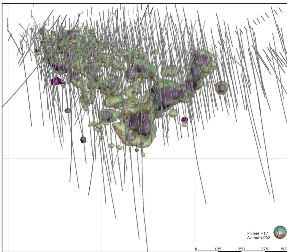
**Figure 13-14: Nickel high-grade (green) and PGE (purple) domain meshes**
