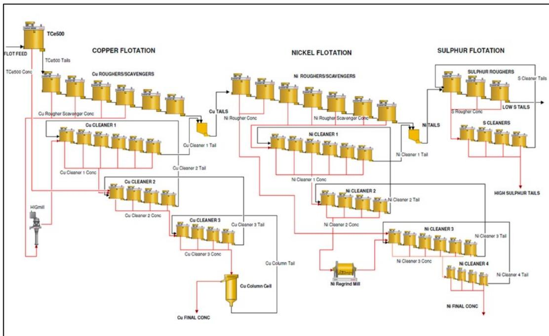
Figure 15-2: Kevitsa Cu and Ni Flotation Circuits (Source: Boliden, 2019)
