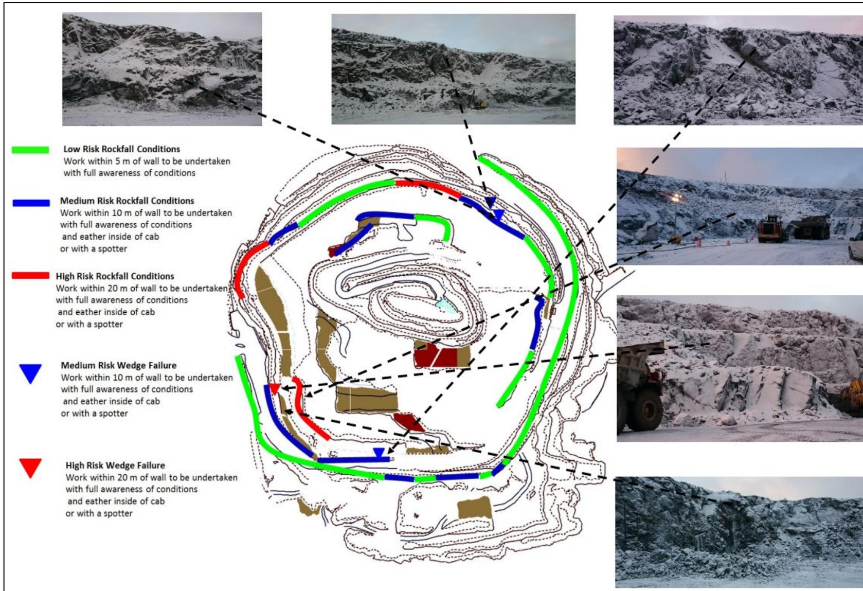
Figure 14-16: Example Hazard Map for Stage 2 and 3 mining at Kevitsa
