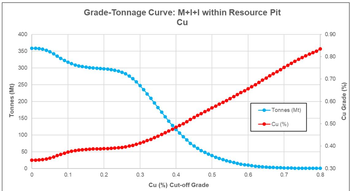
**Figure 13-23: Grade-tonnage curve for total copper in Measured+Indicated+Inferred blocks within the Mineral Resource pit shell**
