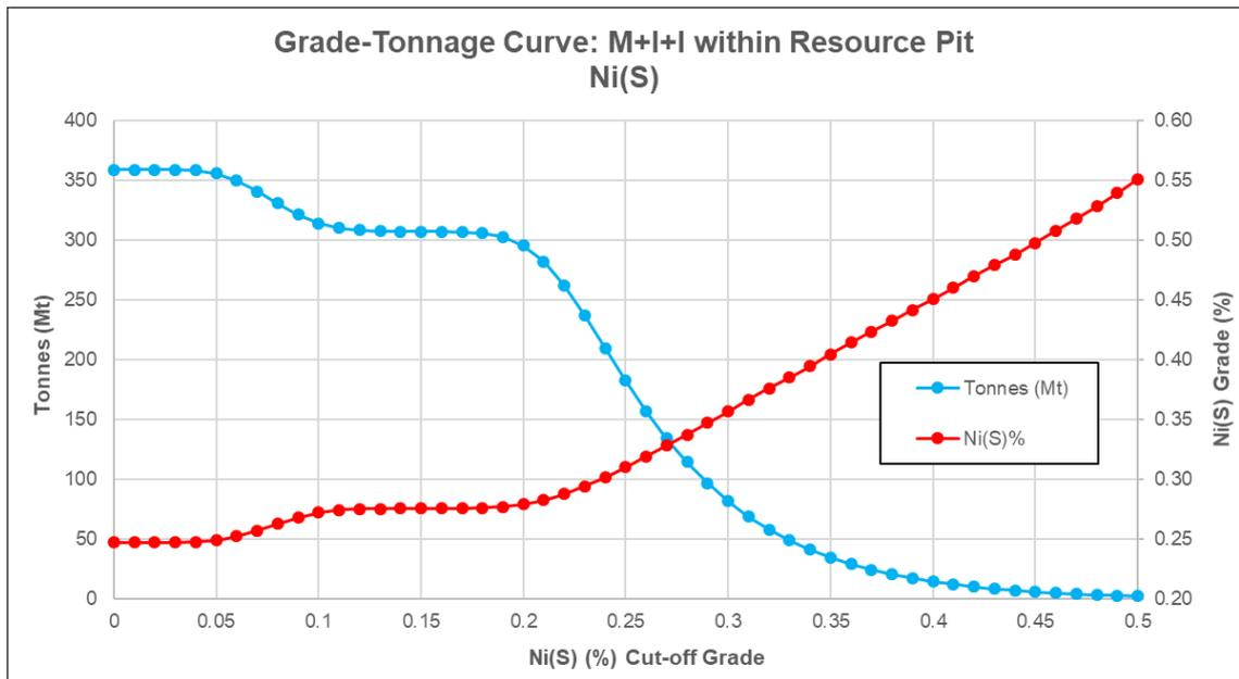
**Figure 13-22: Grade-tonnage curve for sulphidic nickel in Measured+Indicated+Inferred blocks within the Mineral Resource pit shell**
