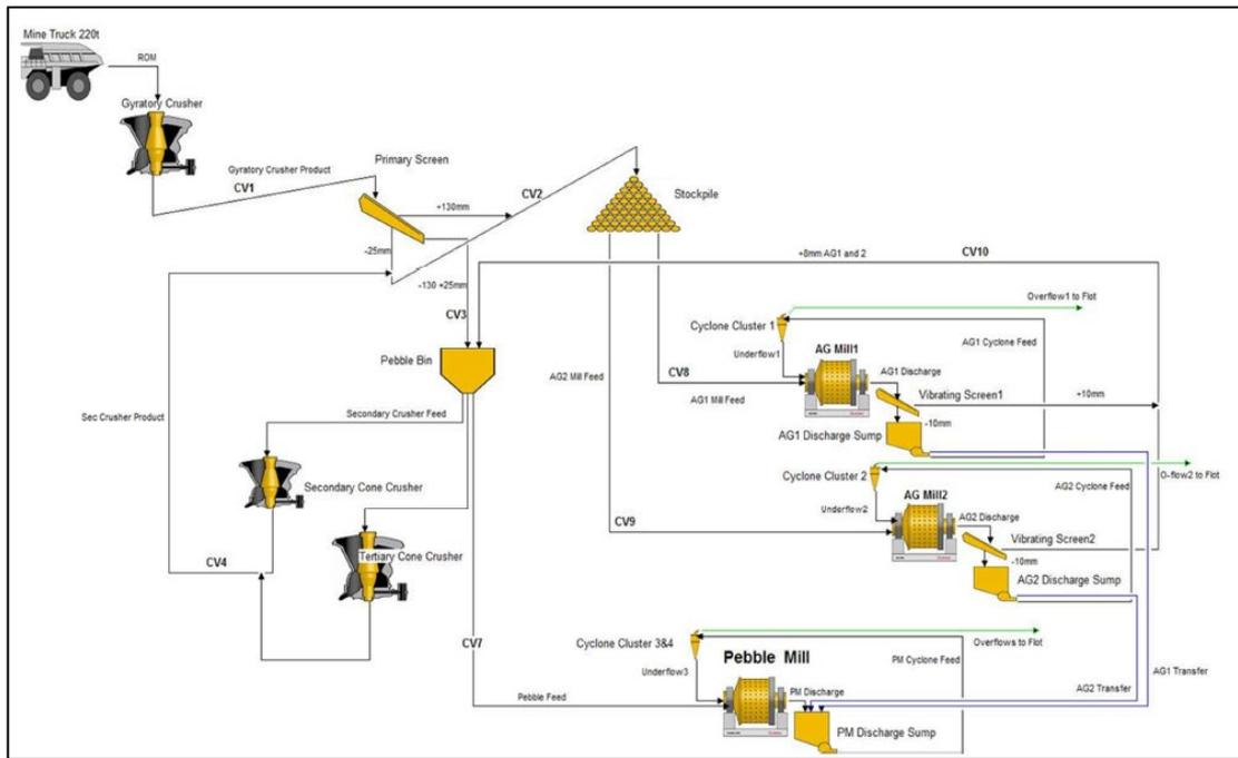
Figure 15-1: Kevitsa Crushing and Grinding Circuits (Source: Boliden, 2019)
