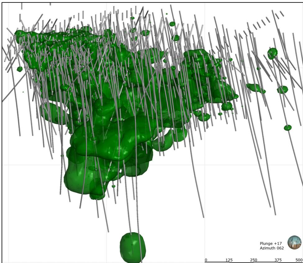
**Figure 13-13: Nickel low-grade domain meshes**
