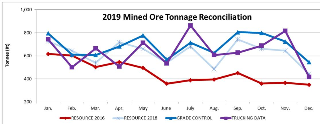
**Figure 13-18: 2019 tonnage of ore mined from MRE 2016 block model, MRE 2018 block model, grade control block model and production (truck)**
