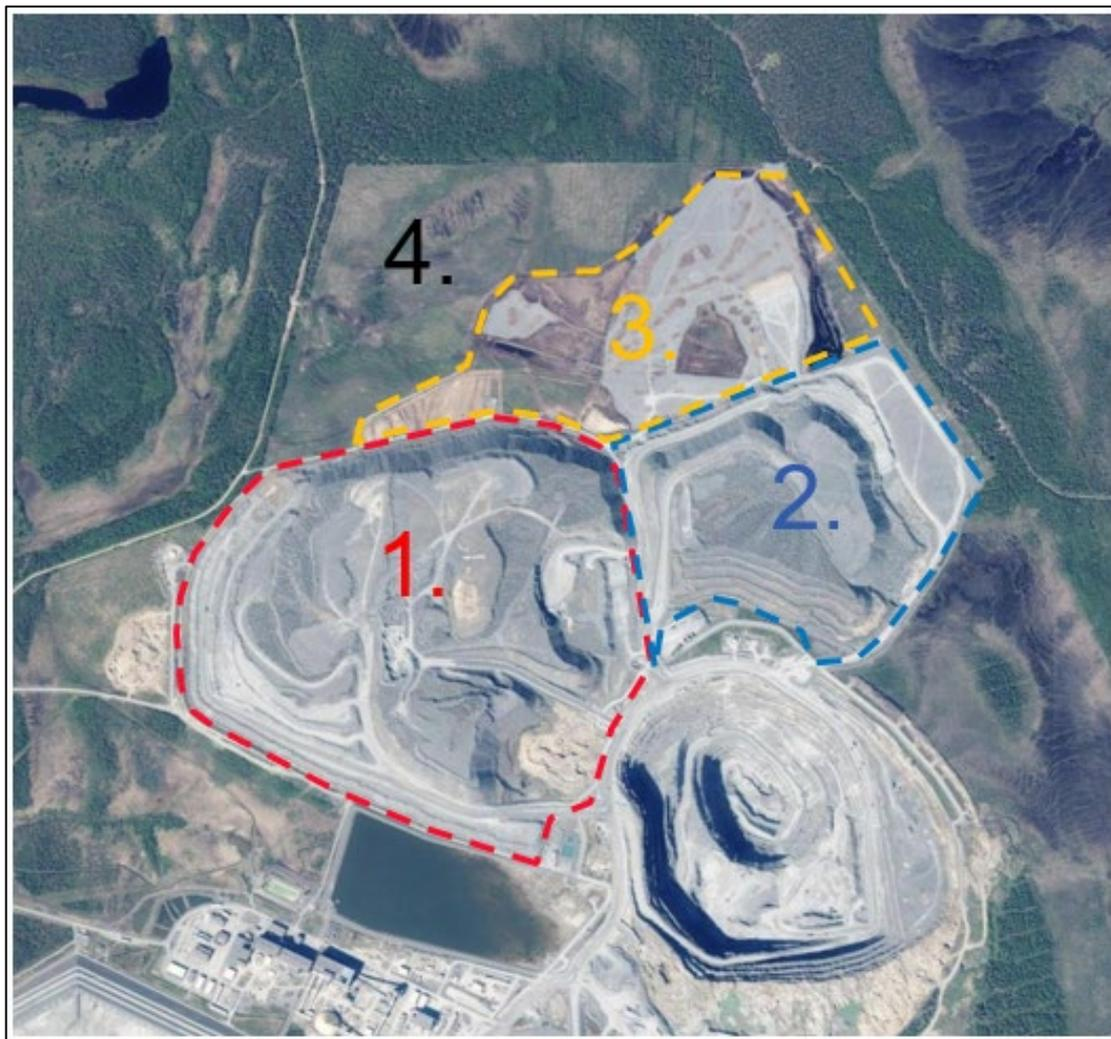
Figure 14-9: Waste dump locations for the Kevitsa mine
