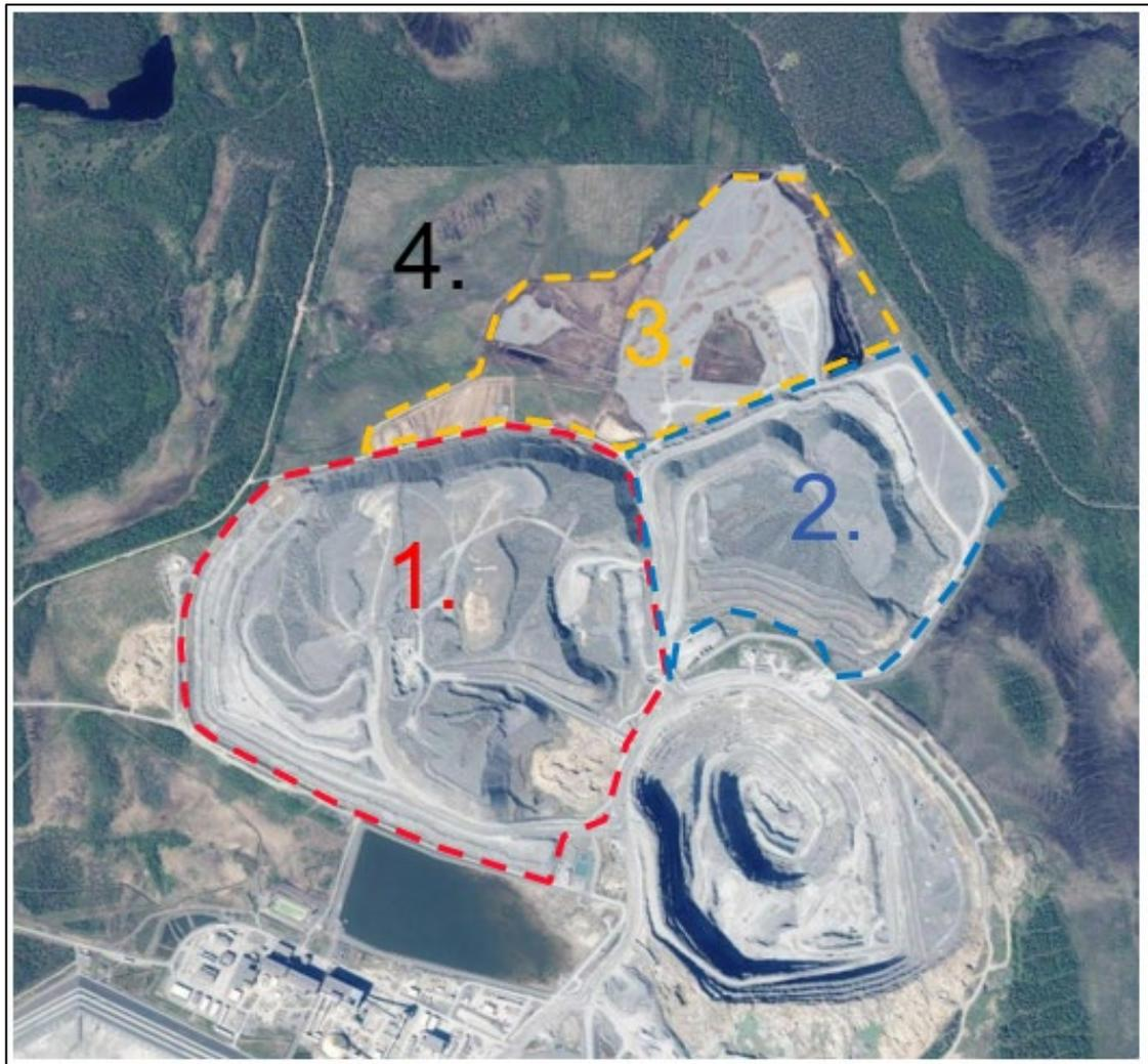
**Figure 14-9: Waste dump locations for the Kevitsa mine**
