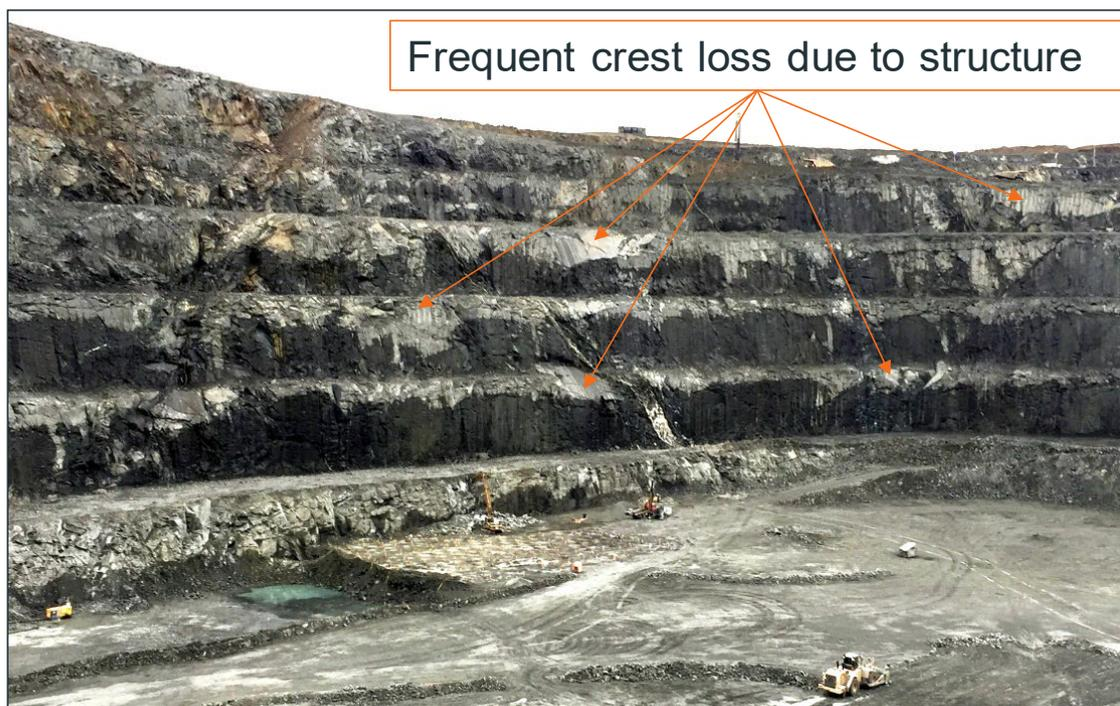
**Figure 14-15: Example of frequent bench scale crest loss to structure**
