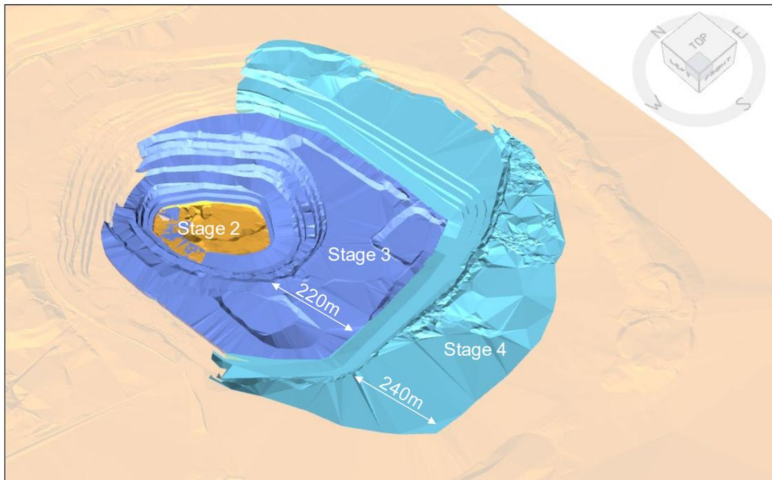
**Figure 14-5: Kevitsa pushbacks solids (Stage 2, 3, & 4)**
