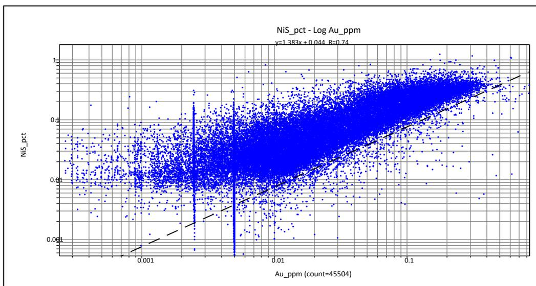
**Figure 13-9: Scatterplot showing Au (ppm) vs Ni(S) %**
