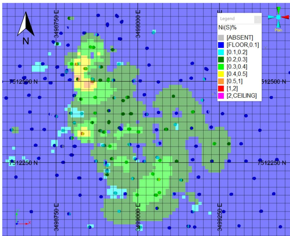
Figure 13-15: Plan view (-100 m Z) of Ni(S) estimate block model and sample composites (section thickness 10 m)
