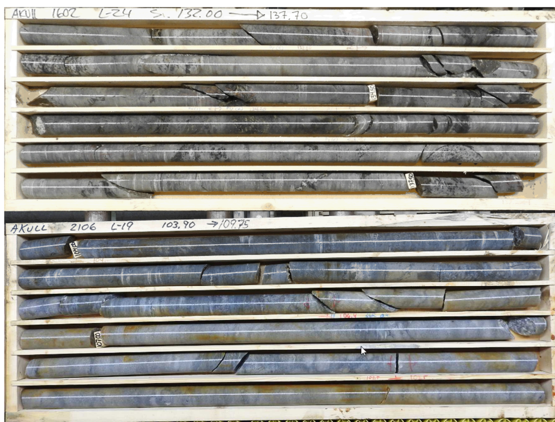
Figure 16: High-grade gold intersections, which are typical boxes of Kankberg mineralised core. Hole ID, box number and from-to depths are shown.
