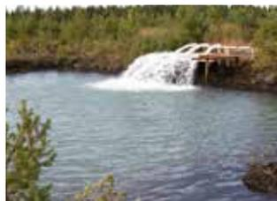
**Kedträsk, September 2012.** While draining the open-pit mine, the water was limed a number of times. The water was collected in settling ponds so that the sludge could be dealt with and the water quality controlled.
