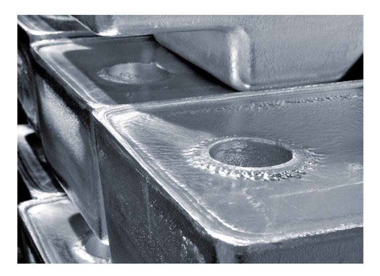
ZINC-BRIGHT®, a zinc-bismuth-tin alloy for Lead-free galvanizing, was developed by Boliden to meet the needs of our customers in the general galvanising industry. The easy to use, ready-made alloy means no more mixing of different components, saving our customers time, effort and costs.
