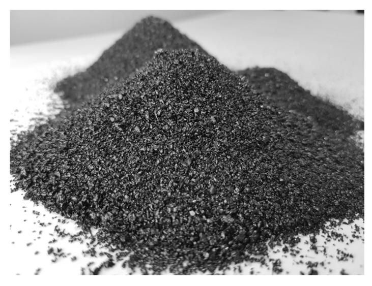
**IRON SAND** is a glassy iron silicate aggregate consisting of granulated slag, extracted as a by-product from Boliden Rönnskär's copper production.
