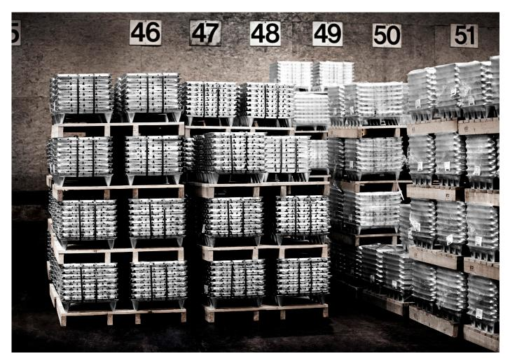
**ZINKAL 5 AND ZINKAL 10,** two Zinc – Aluminium master alloys with respectively 5 or 10%Al, have been specially developed to meet the needs of our customers in the general galvanizing industry.
