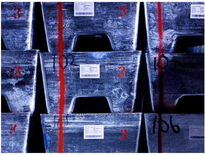
**ZINIGAL PLUS®**, a zinc-nickel alloy containing bismuth, was developed by Boliden to meet the needs of our customers in the general galvanising industry. The easy to use, ready-made alloy means no more mixing of different components, saving our customers time, effort and costs.
