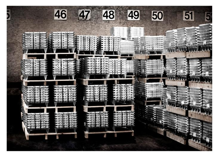
**NORZAK** is a Zinc-based die-cast-alloy especially developed for hot chamber die-casting. The applied Aluminium-concentration grants best fluidity and excellent impact strength.
