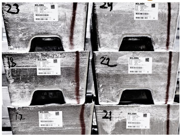
**MAGIGAL** is family of zinc-aluminum-magnesium alloys developed by Boliden together with the steel industry to meet the needs of our customers in continuous hot dip galvanizing.
