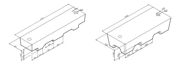
**Jumbo 2,000 kg** 1,920 ± 100 kg 2,130x490x365 (± 6 mm) **Jumbo 1,400 kg** 1,450 ± 100 kg 1,430x565x330 (± 6 mm)
