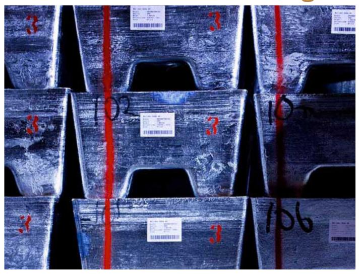
**ZINIGAL®**, a zinc-nickel alloy, was developed by Boliden to meet the needs of our customers in the general galvanising industry. The easy to use, ready-made alloy means no more mixing of different components, saving our customers time, effort and costs.
