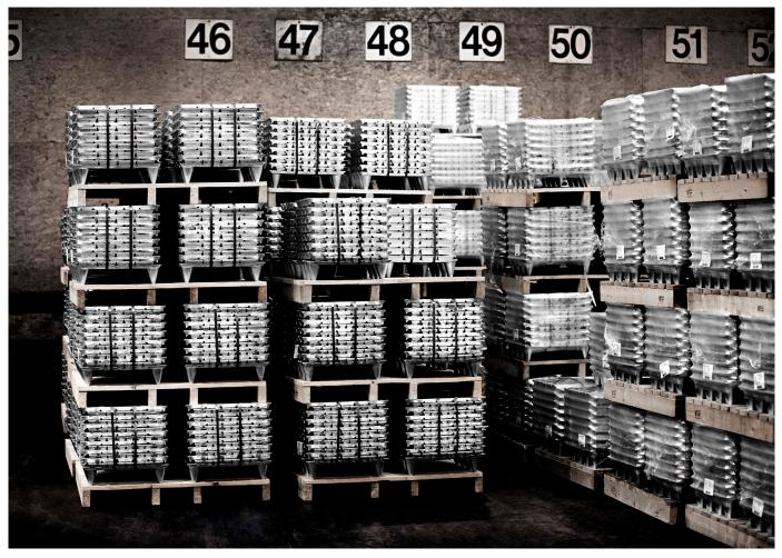
**NORZAK** is a Zinc-based die-cast-alloy especially developped for hot chamber die-casting. The applied Aluminiumconcentration grants best fluidity and excellent impact strength.
