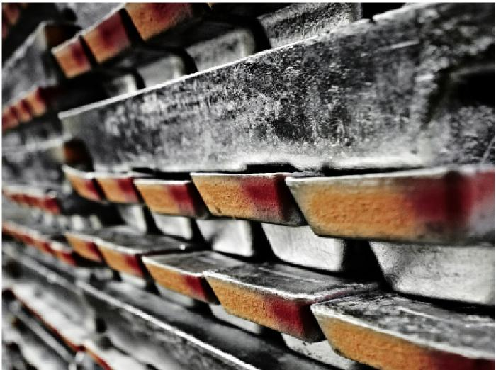
**REFINED LEAD INGOTS** are produced from scrapped batteries and other lead-containing recyclables at Bergsöe, one of Boliden's five smelters, located in Landskrona Sweden. The smelter is the only secondary lead smelter in the Nordics and has a strategic location for sourcing material and serving customers in Europe. Bergsöe has a production capacity of approximately 50,000 metric tonnes lead per year.
