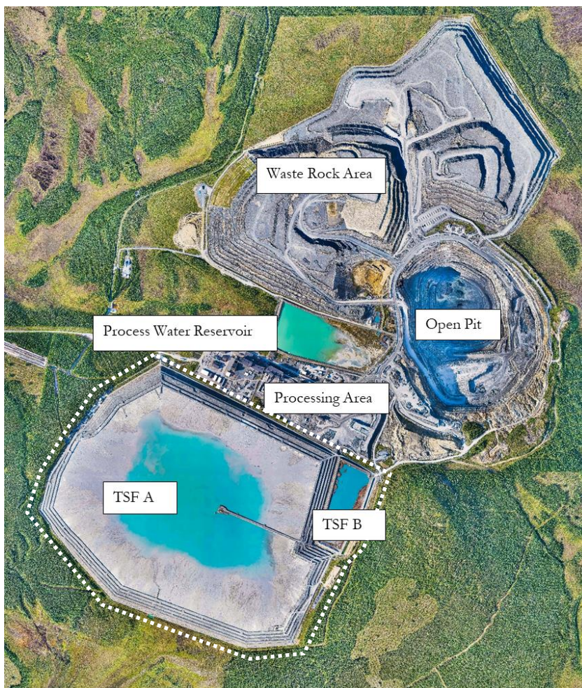
Figure 2 Aerial photo (2022) of the Kevitsa mine – The tailings facility area marked with a dotted line
